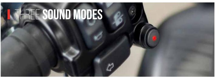
Dr. Jekill & Mr. Hyde | The Exhaust is a smart exhaust system that gives you the ultimate riding experience. Our electronically adjustable system allows riders to control the exhaust with a push of the button mounted on the handlebar. You can choose per situation whether you
